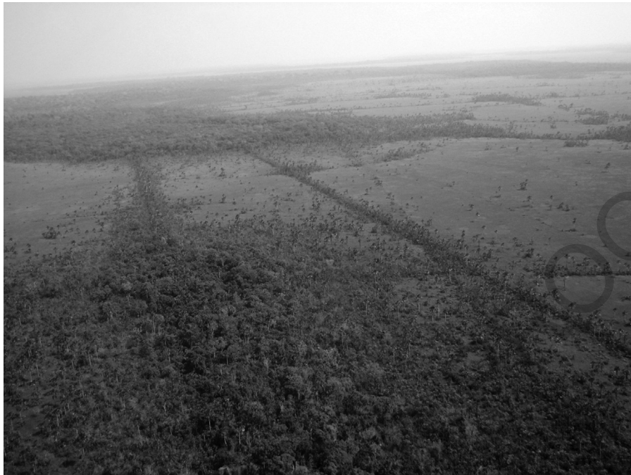
Figure 4.8 Four pre-Columbian causeways and canals connecting forest islands in the Bolivian Amazon. The palm covered causeways are 3 to 4 m wide and 1 m tall with adjacent canals of 2 to 3 m wide and 1 m deep. Baures in 2006. (Clark Erickson)
